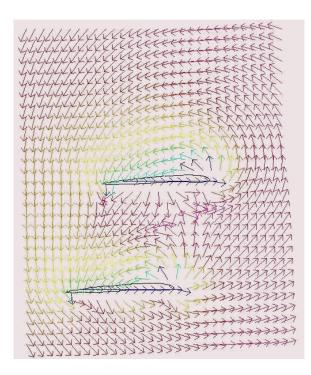
Velocity scans are displayed as arrows oriented with the local flow direction. The color of each arrow indicates the magnitude of one of the plottable parameters, namely Cp, Velocity magnitude, or Mach number. The length of the arrow has no meaning.
