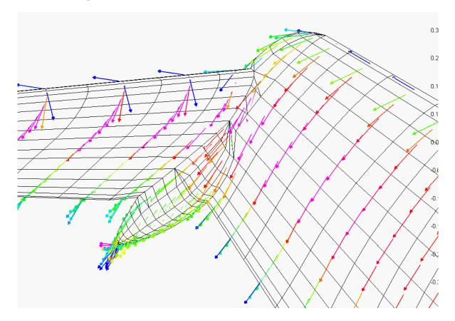
The direction of the arrow indicates the orientation of the local flow. The color of the arrow indicates the flow speed, pressure or Mach number. Arrow length indicates nothing, but can be adjusted in the *Display* > *Options* dialog under *Vector Display*.
