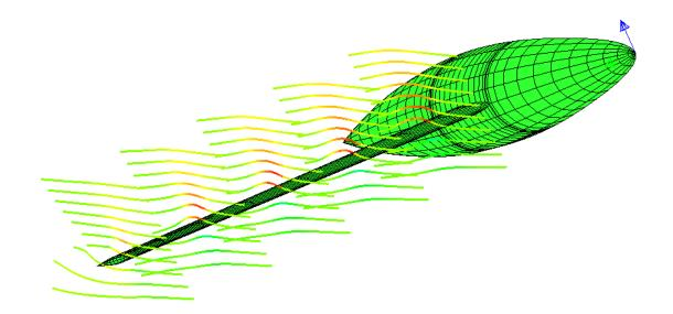
As in the CMARC input file, streamlines are defined by a point of origin, upstream and downstream distances, and the interval between points along the streamline.
